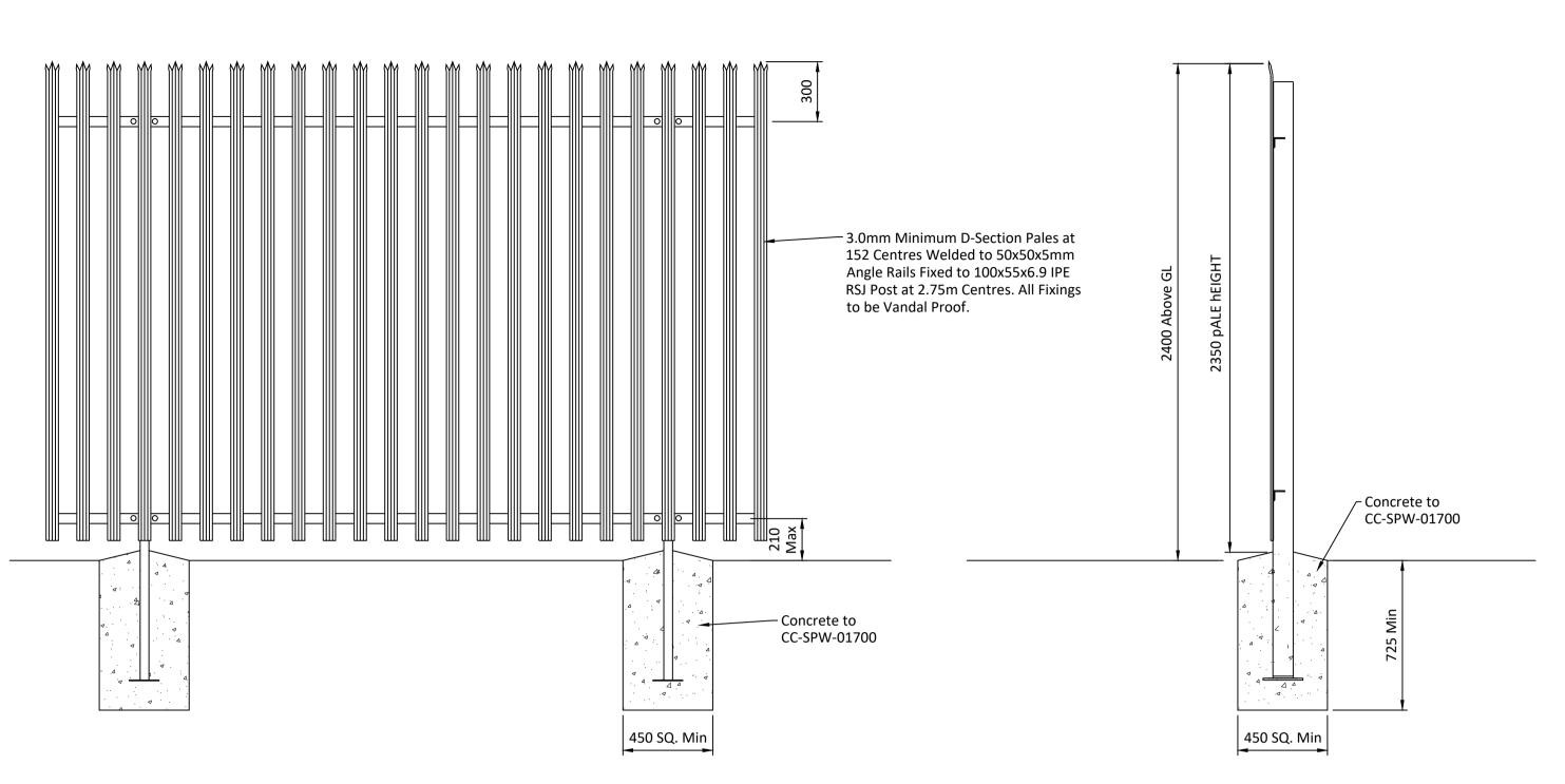
– Palisade Fence 150mm Reinforced Concrete Plinth. 1000
