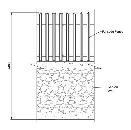
PROPOSED PALISADE FENCE ON GABION WALL **SECTION**
